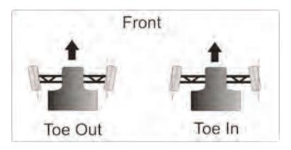
If more grip is needed in the front then you could consider adjusting toe out to a maximum of 10mm. Make sure that the balance of the kart is not upset too much if you do this though. Normally the water on the track must be very wet before toe out is used.
